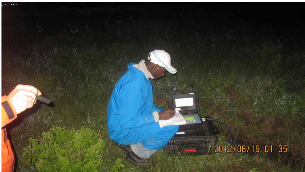
Fig. 5. NAWASSCO staff taking minimum night flow measurements at NAKA.
